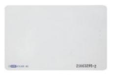
The iClass 2k/2 card from HID is a 13.56 MHz contactless smartcard designed for use with HID's door access control systems plus other compatible applications. The card contains 256 bytes (2k bits) of memory and is configured with 2 application areas. The first area stores the HID card number and the other is customisable for user requirements.
